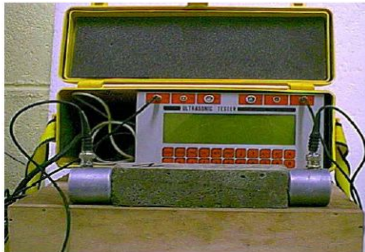
Standard E0641 Ultrasonic test setup
