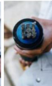
Technora 9-bar tendon in a stainless steel bonded anchorage.
