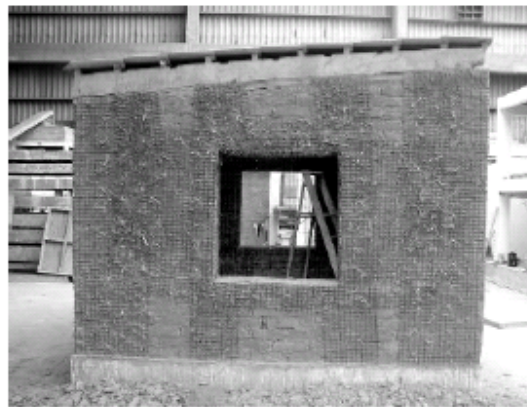
External geogrid mesh reinforcement (75% of walls covered)
