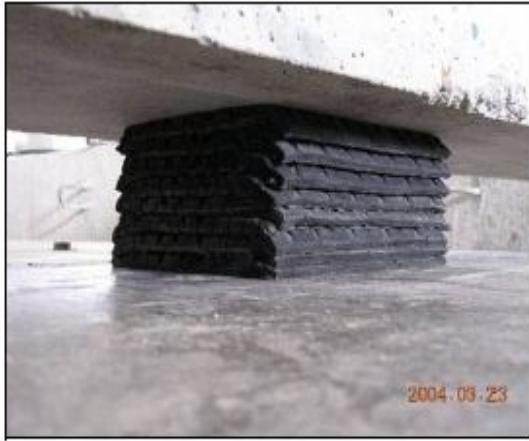
Preparation of scrap tire pad (STP)
