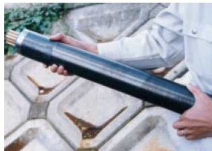
Technora 9-bar tendon in a stainless steel bonded anchorage.
